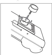
After attaching the belt clip and the shoe mount adapter, insert the microphone stand adapter into the screw hole at the top of the shoe mount adapter, and then rotate the microphone stand adapter until it is securely attached.
